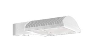
Specification Grade Area lights with multi-level motion sensor available in IES Type II distributions. For use in parking lots, roadways, pathways and general area lighting. Mounts to 4" square steel poles at 15-25'. Designed to replace 250W Metal Halide Area Lights. Patent Pending thermal management system. 5 Year Warranty.
