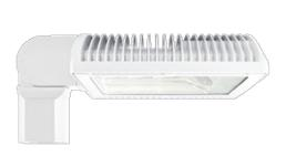
Specification Grade Area lights available in IES Type II distributions. For use in parking lots, roadways, pathways and general area lighting. Mounts to 4" square steel poles at 15-25'. Designed to replace 250W Metal Halide Area Lights. Patent Pending thermal management system. 5 Year Warranty.
