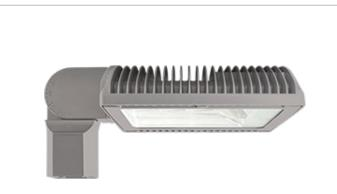
Specification Grade Area lights available in IES Type II distributions. For use in parking lots, roadways, pathways and general area lighting. Mounts to 4" square steel poles at 15-25'. Designed to replace 250W Metal Halide Area Lights. Patent Pending thermal management system. 5 Year Warranty.
