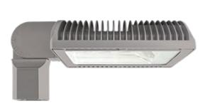
Specification Grade Area lights available in IES Type II distributions. For use in parking lots, roadways, pathways and general area lighting. Mounts to 4" square steel poles at 15-25'. Designed to replace 250W Metal Halide Area Lights. Patent Pending thermal management system. 5 Year Warranty.
