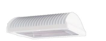
Specification grade area lights available in IES Type IV distributions. Suited for mounting on the sides of buildings and walls, and for illuminating the perimeter of parking areas. Mounts to 4" square steel poles at 20-35'. Patent pending management system. 5 Year Warranty.
