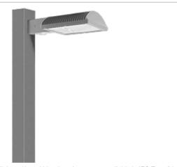
Specification grade area lights with multi-level motion sensor available in IES Type IV distributions. Suited for mounting on the sides of buildings and walls, and for illuminating the perimeter of parking areas. Mounts to 4" square steel poles at 20-35'. Patent pending management system. 5 Year Warranty.
