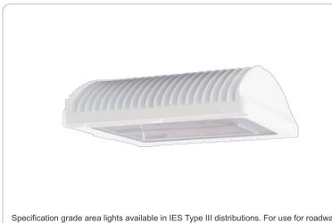
Specification grade area lights available in IES Type III distributions. For use for roadway, general parking and other area lighting applications where a larger pool of lighting is required. Mounts to 4" square steel poles at 20-35'. Patent pending thermal management system. 5 Year Warranty.
