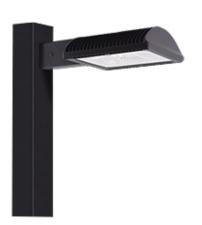
Specification grade area lights available in IES Type III distributions. For use for roadway, general parking and other area lighting applications where a larger pool of lighting is required. Mounts to 4" square steel poles at 20-35'. Patent pending thermal management system. 5 Year Warranty.
