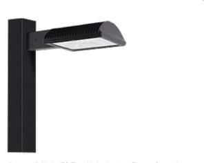
Specification grade area lights available in IES Type III distributions. For use for roadway, general parking and other area lighting applications where a larger pool of lighting is required. Mounts to 4" square steel poles at 20-35'. Patent pending thermal management system. 5 Year Warranty.
