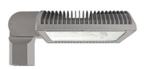
Specification grade area lights available in IES Type III distributions. For use for roadway, general parking and other area lighting applications where a larger pool of lighting is required. Mounts to 4" square steel poles at 20-35'. Patent pending thermal management system. 5 Year Warranty.
