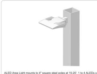
ALED Area Light mounts to 4" square steel poles at 15-20'. 1 to 4 ALEDs can be mounted to each pole. IESNA Full Cutoff, Fully shielded optics. 5 year warranty.
