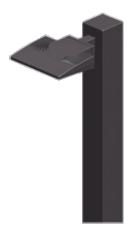
ALED Area Light mounts to 4" square steel poles at 15-20'. 1 to 4 ALEDs can be mounted to each pole. IESNA Full Cutoff, Fully shielded optics. 5 year warranty.
