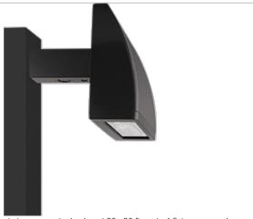
Full Cutoff mounitng. Mounts to square steel poles at 20 - 30 ft, up to 4 fixtures per pole. Patent Pending thermal management system. 100,000 hour L70 lifespan. 5 Year Warranty.
