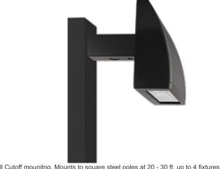
Full Cutoff mouniting. Mounts to square steel poles at 20 - 30 ft, up to 4 fixtures per pole. Patent Pending thermal management system. 100,000 hour L70 lifespan. 5 Year Warranty.
