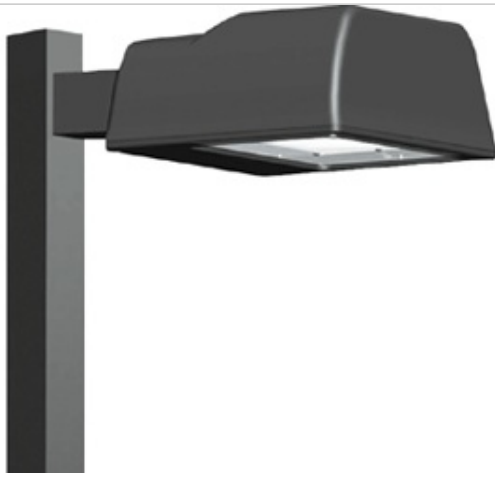
Type II distribution Area Light with pole top fixed arm mount. Fixed mounting at 90° to pole. Drilling 2" on center. Factory wired for 277V. Lamp supplied.
