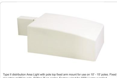
mounting at 90° to pole. Drilling 2" on center. Factory wired for 277V. Lamp supplied. Weight: 14.8 lbs
