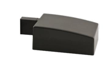
Type II distribution Area Light with pole top fixed arm mount for use on  $10^{\circ}$  -  $15^{\circ}$  poles. Fixed mounting at  $90^{\circ}$  to pole. Drilling 2" on center. Factory wired for 277V. Lamp supplied.
