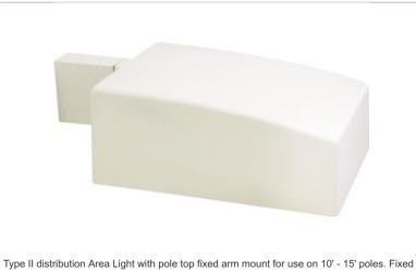
mounting at 90° to pole. Drilling 2" on center. Factory wired for 277V. Lamp supplied. Weight: 20.4 lbs
