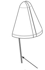
Use UL approved wiring connectors for SPT-1 cord
