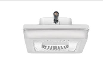
This ultra high efficiency LED garage light delivers up to 118 lumens per Watt. An integrated motion/photo sensor option provides multi-level lighting control. Available in 30, 42 and 55 Watt versions that replace 70 to 175 Watt metal halide fixtures.
