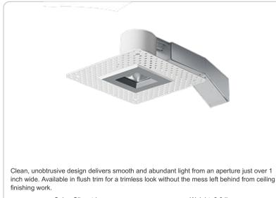
Project: Type: Prepared By: Date: LED Info **Driver Info** Type: Constant Current Watts: 8W 120V: 0.08A Color Temp: 3000K 208V: N/A Color Accuracy: 83 CRI 240V: N/A L70 Lifespan: N/A 277V: N/A Lumens: 567 Input Watts: 9W Efficacy: 65 LPW Efficiency: 91%
