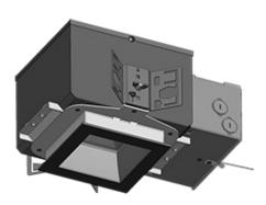
Easy to install 4" and 6" rough-in with die-cast aperture ring, removable driver, thermal protector and adjustable butterfly brackets. This rough-in is designed to make new construction recessed downlighting easy 90 CRI.
