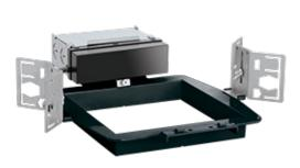
Easy to install 4" and 6" rough-in with die-cast aperture ring, removable driver, thermal protector and adjustable butterfly brackets. This rough-in is designed to make new construction recessed downlighting easy 90 CRI.
