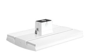
LED High Bay fixture ideal for large indoor spaces, including warehouses, gymnasiums and distribution centers that require mounting heights from 15 to 50 feet. An integrated motion/photo sensor option provides multi-level lighting control. Available in 95, 150, 185 and 225 Watt versions with equivalencies from 200 to 400 Watt metal halide fixtures.
