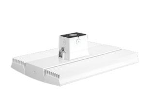
LED High Bay fixture ideal for large indoor spaces, including warehouses, gymnasiums and distribution centers that require mounting heights from 15 to 50 feet. Available in 95, 150, 185 and 225 Watt versions with equivalencies from 200 to 400 Watt metal halide fixtures.
