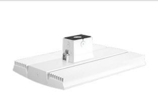
LED High Bay fixture ideal for large indoor spaces, including warehouses, gymnasiums and distribution centers that require mounting heights from 15 to 50 feet. Available in 95, 150, 185 and 225 Watt versions with equivalencies from 200 to 400 Watt metal halide fixtures.
