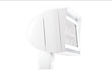
Ultra high output, high efficiency LED floodlight with wide NEMA type 6H x 6V beam spread. Patent Pending airflow technology ensures long LED and driver lifespan. Use for general and security lighting for large areas, building facades, signs and landscapes.
