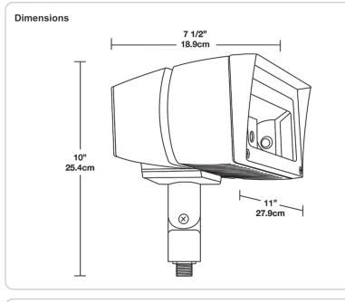
**Ordering Matrix** Family Watts Mount Color Temp Beam Spread Finish Dimming Photocell **FFLED** 80 = 80W = Arm = Cool  $= 7H \times 6V$ = Bronze = No Dimming = No Photocell T = Trunnion Y = Warm **B44** = 4H x 4V W = White /D10 = Dimmable /PC = 120V Button SF = Slipfitter N = Neutral B55 = 5H x 5V /PC2 = 277V Button /PCS = 120V Swivel /PCS2 = 277V Swivel
