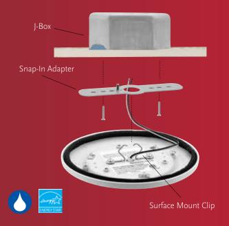
The surface mount uses an intuitive snap-in system that makes surface mount installation easier than ever. Simply install the snap-in-adapter onto the junction box and connect wires. To finish the installation, snap the fixture into place using the surface mount clip. A great solution for fire rated applications when used in conjunction with a fire rated j-box.
