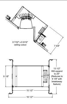
Real Nail® 3 Bar Hangers Telescoping Real Nail® 3 system permits quick placement of housing anywhere within 24'O.C. joists or suspended ceilings • Includes removable nail for repositioning of fixture in wood joist construction • Integral T-bar mounting feature for suspended ceilings • Design covered under US Patent D552,969.
