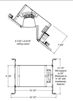
Mounting Frame 22-gauge die-formed galvanized steel mounting frame • Rough-in section (junction box, mounting frame, housing and bar hangers) fully assembled for ease of installation.
