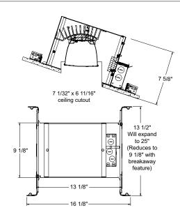
Mounting Frame 22-gauge die-formed galvanized steel mounting frame • Rough-in section (junction box, mounting frame, housing and bar hangers) fully assembled for ease of
