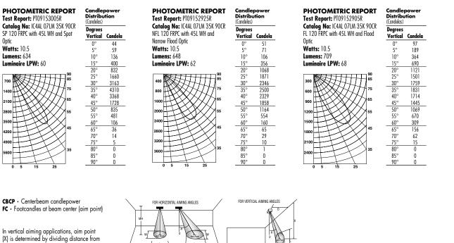
In vertical aiming applications, aim point (X) is determined by dividing distance from the wall (D) by the tangent of the desired aim angle (A) (0.5774 for 30°, 1.0 for 45°).
