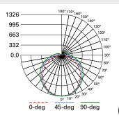
**4APVTLD-SL3C3** Electronic Driver Linear LED 4000K Spacing criterion: (II) 1.23 x mounting height, (⊥) 1.3 x mounting height Lumens: 4620 Input Watts: 31.6W Efficacy: 146 Im/W Test Report: 4APVTLD-SL3C3-MID-4000K-120V.IES
