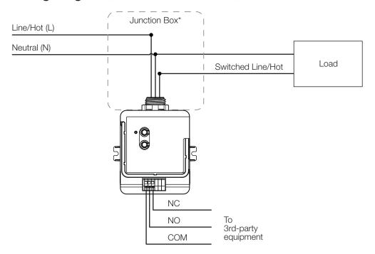
\* NOTE: Some applications (in U.S.A.) require the PowPak module to be installed inside an additional junction box. For information about how to perform this installation, please see Application Note #423 (P/N 048423 at www.lutron.com). Please consult all local and national electric codes for proper installation methods.
