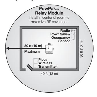
All Wireless Transmitters must be installed within 30 ft (10 m) of the PowPak $_{\text{TM}}$  Relay Module.
