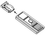
Remove existing battery and replace with a new CR 2032 battery, positive (+) side down. Slide battery holder back into the Pico Control until it snaps into place.
