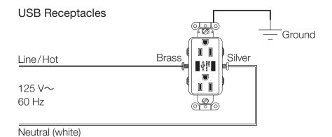
**Note:** Top and bottom receptacles cannot be split apart into independent Line/Hot and Switched Hot connections.
