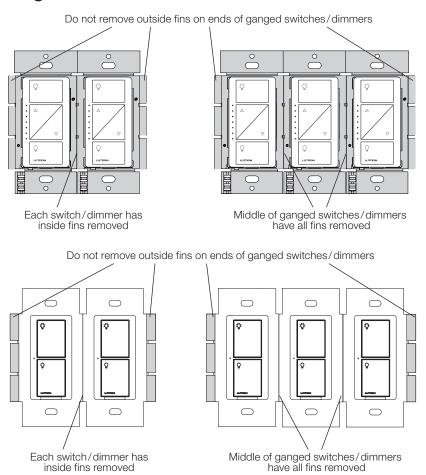
Note: Fin removal is not required for PD-5WS-DV, as it ships without fins.
