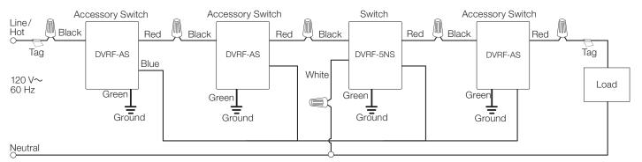
Up to ten (10) accessory switches may be connected to the switch. Total blue wire connection wire length may be up to 150 ft (45 m).
