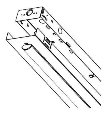
• Install using provided tek screws through mounting bracket, as shown.
