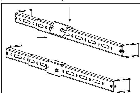
Figure 2: Connect plastic attachment on the joist bar as shown on outside part of the bar (joist bar can only be used for 4" and 6" version of LED Wafer).
