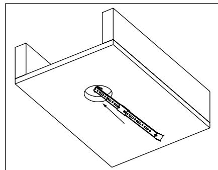
Figure 3: Insert joist bar through the ceiling cut-out hole making sure both ends of the bar touch each side of the joist.
