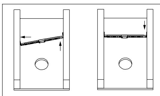
Figure 4: Slam one side of the joist bar against one side of ceiling joist and push up other side of joist bar up and against other ceiling joist and pull it down until it is secured (make sure joist bar is secured high enough so junction box can be held securely).
