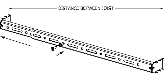
Figure 1: Measure the joist distance and adjust joist bar accordingly as shown. Use screwdriver (not included) to insert plastic fastener into joist bar to lock it in place.
