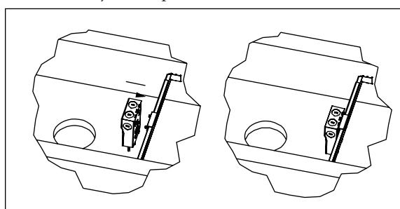
Figure 5: Connect junction box to luminaire using cable connector and connect junction box wire to wires from power supply. Attach junction box to the plastic attachment on joist bar through the junction box keyhole as shown and install luminaire through the ceiling hole.
