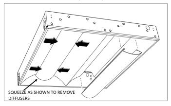
Figure 3: Diffuser Removal/Installation
