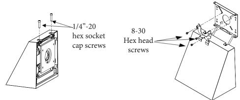
2. Position the wall mounting plate over the j-box. Attach the plate to the j-box using screws that came with the j-box. (see the chart on the next page for fixture weights)
