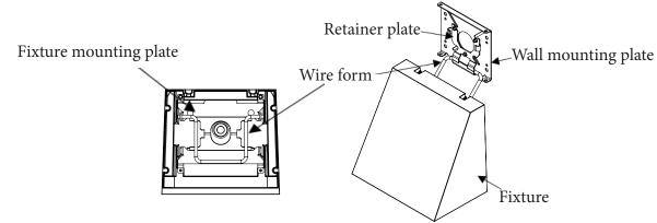
1. Use the 3/16" allen wrench or hex key to detach the wall mounting plate from the fixture by removing the 1/4"- $20 \times 1$  hex socket cap screws (x 2).
