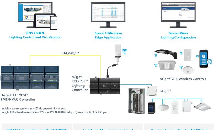
HVAC Integration with ECLYPSE and Third Party Controllers Lighting Management and Control Through Web Applications Connection with nLight Wired and nLight AIR Devices
