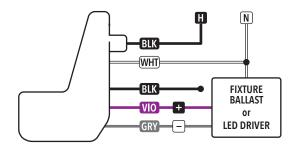
Line Voltage Interchangeable Lens Fixture Mount: 2P w/ Single Zone On/Off Photocontrol
