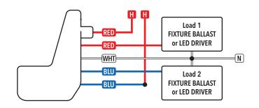
Line Voltage Interchangeable Lens Fixture Mount: 2P w/ Single Zone On/Off Photocontrol (HVOLT) Line Voltage Interchangeable Lens Fixture Mount: 2-Phase (HVOLT)
