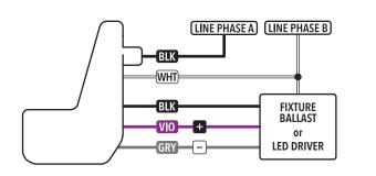
Line Voltage Interchangeable Lens Fixture Mount (HVOLT)
