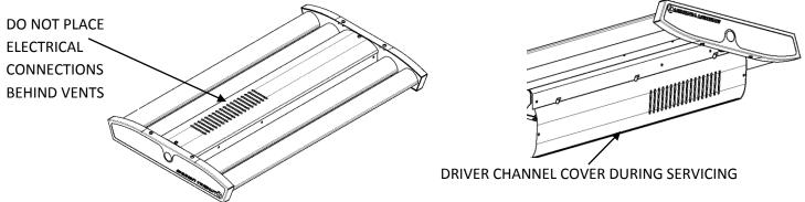
7) Make any necessary adjustments or driver changes. DO NOT PLACE ELECTRICAL CONNECTIONS ABOVE DRIVER CHANNEL COVER VENTS
