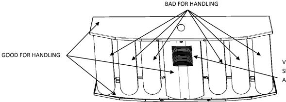
VENT HOLES, DO NOT PUT SPLICE CONNECTIONS ABOVE VENT HOLES
