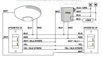
**Note 1:** SPODM (SA) 3X D units should only be used in multi-way applications with SPODM (SA) 3X units (non-dimming) as dimming levels are not communicated between devices.
