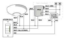
**Note**: If sensor also has dimming output (e.g., CM 9 ADC), connect sensor VIO wire to SPODM and ballast/driver VIO wire. Lowest output level always takes precedence. If no sensor is used, connect the SPODM white wire to the red wires.
