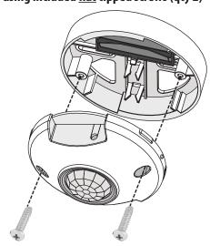
Note: Install decorative sensor lid by pushing up and rotating clockwise.
