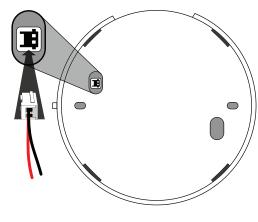
4. Screw sensor to battery extension ring using included flat tipped screws (qty 2)
