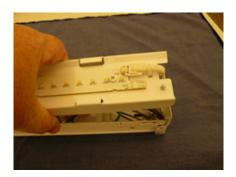
(For continuous row mounting) Remove end plates from adjoining channels and slide row aligner into end of channels and secure with screws.
