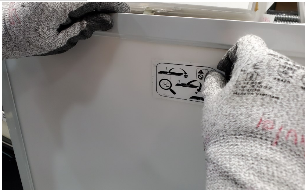
Figure 16: Remove label before RES7 installation
